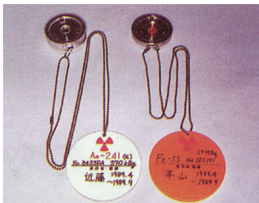
Figure 8-3: Radioactive sources with a tag; white and yellow tags are connected to checking sources and RI, respectively.
