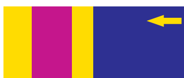
Radioactive water pipe
