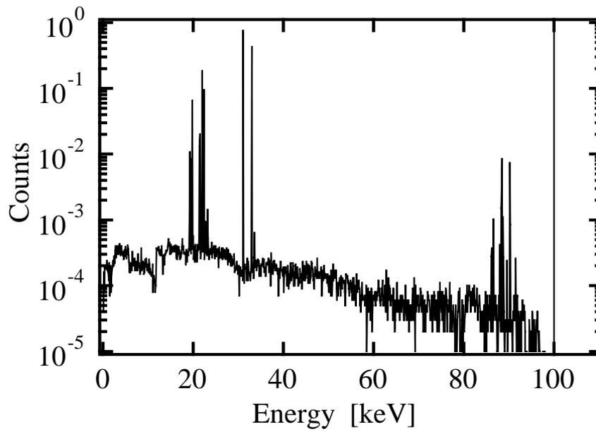
Figure 2: The absorbed energy spectrum for 64-segmented absorbers for X-rays of 100 keV.
