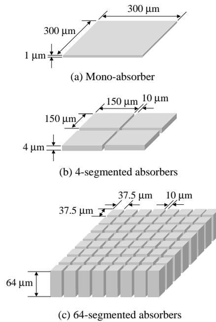
Figure 1: The schematic diagram of a method to divide an absorber into segments.
