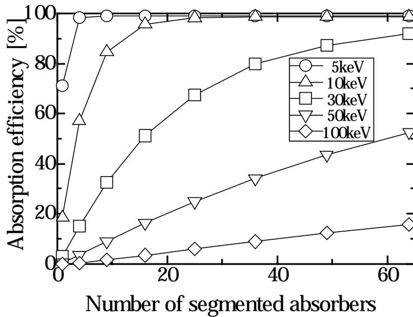
Figure 3: The X-ray absorption efficiency as a function of the number of segmented absorbers. The values of the number of segmented absorbers are equal to the thicknesses of each segmented absorber in  $\mu\text{m}$ .
