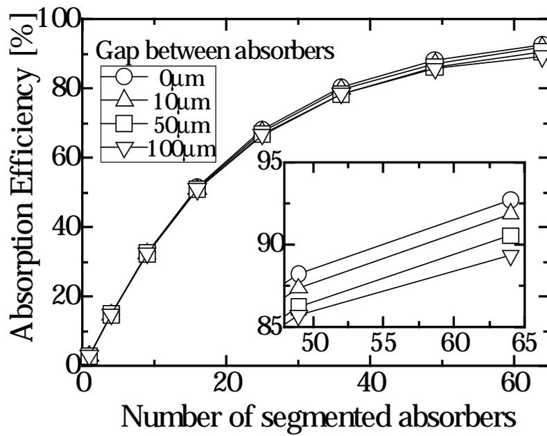
Figure 4: The X-ray absorption efficiency as a function of the gap between segmented absorbers. The incident energy is 30 keV.
