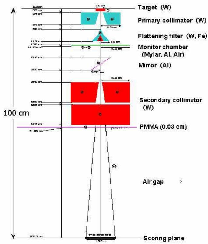
Figure 3 Accelerator model used for the trial calculation.
