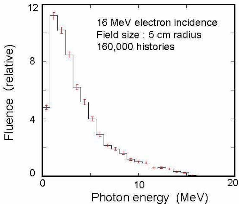
Figure 4 Photon energy spectrum calculated using the accelerator model in Figure 3.
