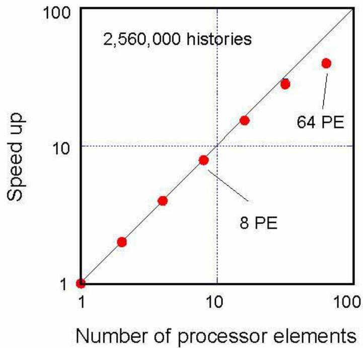
Figure 5 Speed-up of the irradiation fluence calculation due to parallel computing.
