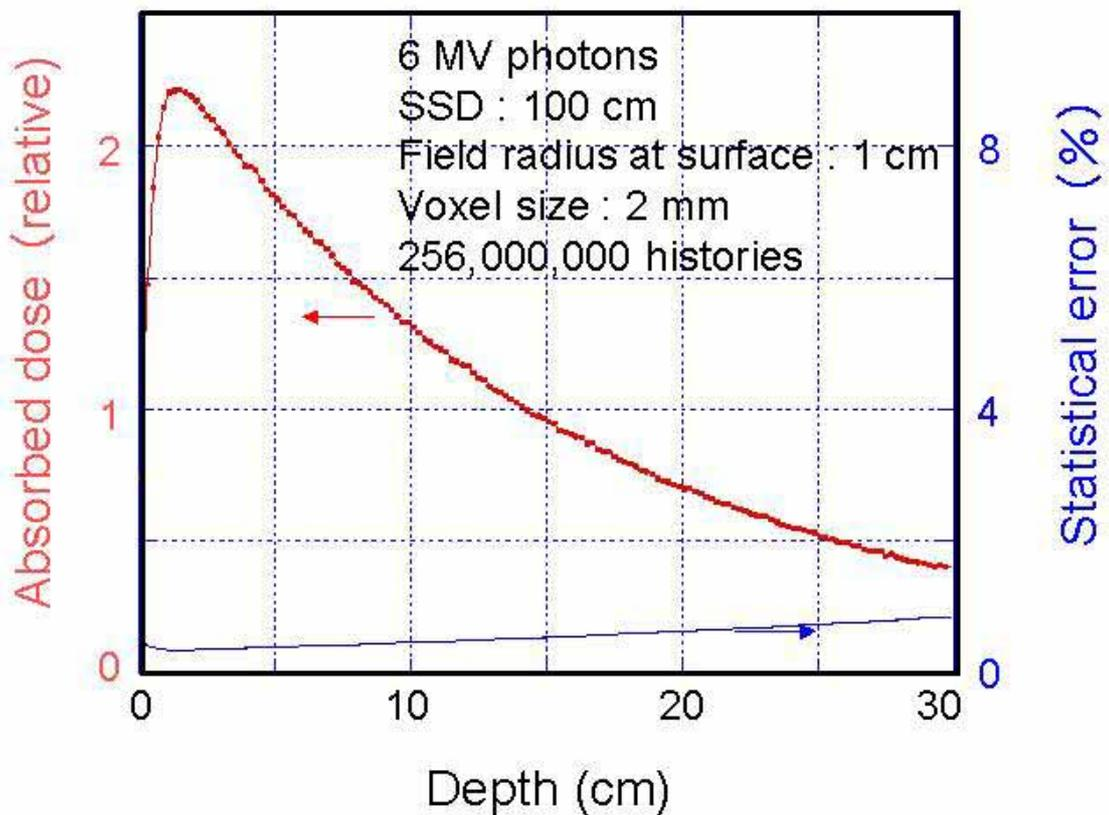
Figure 6 Dose distribution in a water phantom calculated by the prototype of the dose calculation module.
