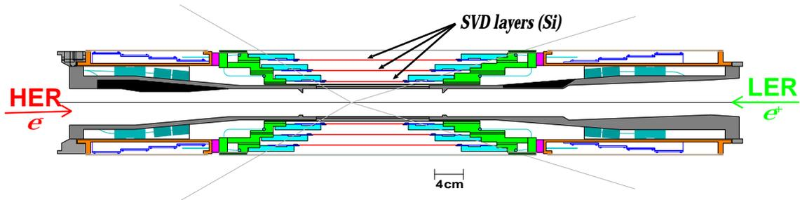
Figure 1: A cross section of the Belle SVD (version 1.4).
