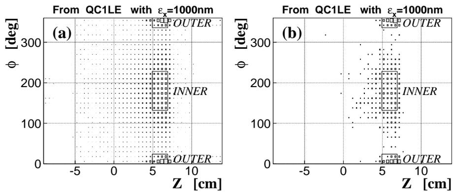
Figure 3: Examples of dose distributions in the SVD first layer (a) with and (b) without the mapping table. The  $Z$  axis is defined as an opposite direction of the LER ( $e^-$ ) beam. 'INNER' ('OUTER') corresponds to the inner (outer) region of the KEKB rings.
