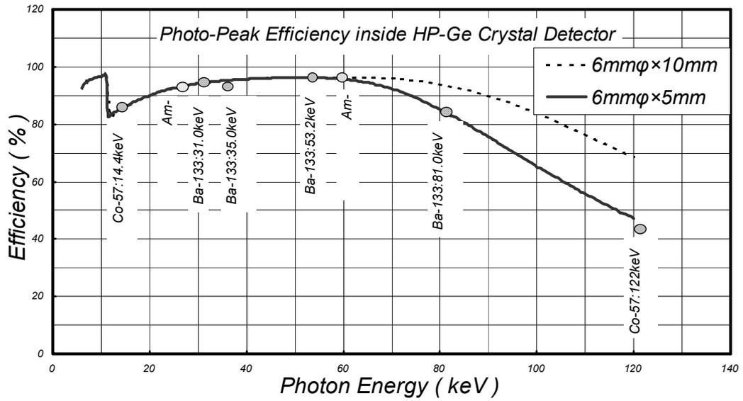
Figure 4: The photon energy efficiency inside the HP-Ge detector (6 mmφ× 5 mm, 6 mmφ× 10 mm).
