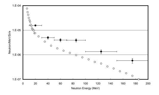
Figure 2: Preliminary results of neutron spectra toward 90 degrees from 2-cm-thick Pb target irradiated by 1.2 GeV electrons. Full circle: Measured at the ATF. Open circle: Calculated using EGS4/PICA3[5]/LAHET2.7[6].
