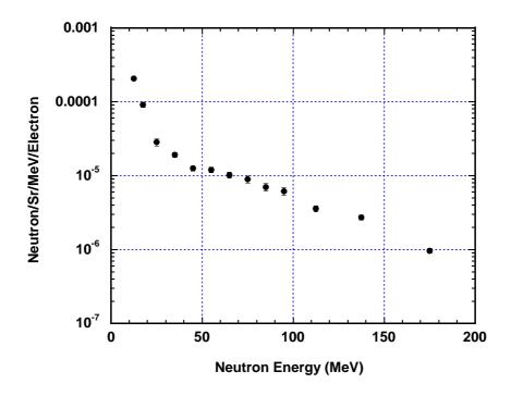
Figure 4: Measured neutron spectra toward 90 degrees from 5.5-cm-thick Pb targets irradiated by 2.04 GeV electrons.
