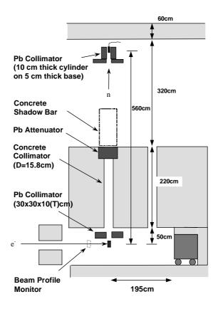
Figure 3: Experimental setup at PAL when 2.04 GeV electrons irradiated Pb targets[3,4].
