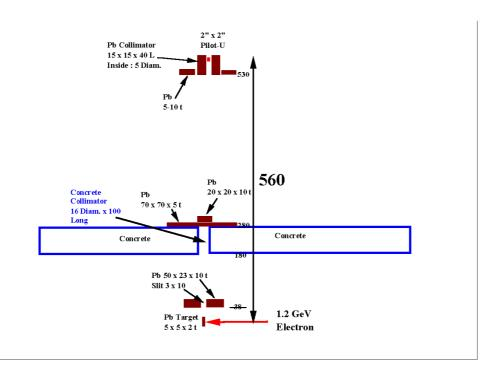
Figure 1: Experimental setup at the ATF when 1.2 GeV electrons irradiated 2-cm-thick Pb target.
