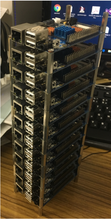
Figure 3: 12 single board computers are connected in one tower. The configuration of PIs is prepared 1 tower of 12 Banana Pi nodes and the other tower of 11 Banana Pi + 1 Raspberry Pi nodes.
