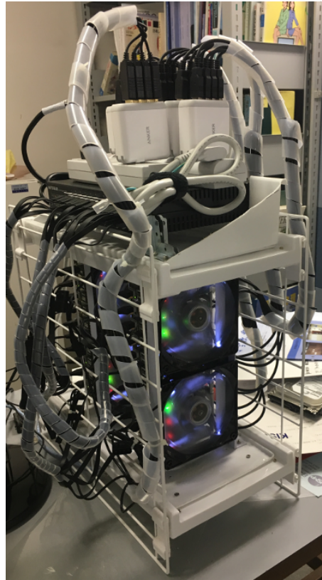
Figure 4: Overall picture of PIs. PIs is configured with 2 towers in Fig. 3, 4 fans (2 per 12 boards), a 24 port switching hub, 5 V USB chargers, power strips, power cables and LAN cables. Fans are necessary for cooling the entire device.
