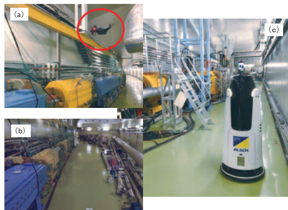
Fig. 2. a) Drone test in the MR tunnel. b) Video from the drone. c) Robot demo in the MR tunnel.
