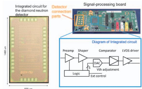
**Fig. 3.** Integrated read-out circuit of the diamond sensor.
