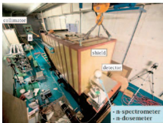
Fig. 2. Experimental setup for 250 cm thick concrete.
