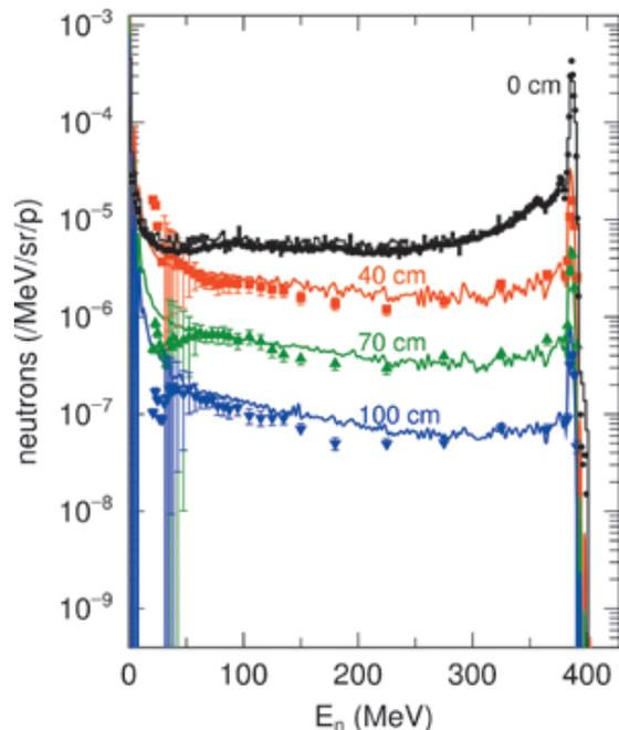
Fig. 3. Neutron energy spectra measured (points) and calculated (lines) behind Fe shielding blocks of different thicknesses.
