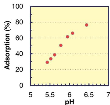
**Fig. 4.** Adsorption (%) of Be(II) on CuO nanoparticles in water as a function of pH. CuO nanoparticles (Average size: 48 nm) : 0.50 g; Water: 20 ml.
