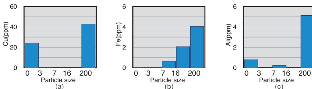
**Fig. 3.** Non-colloidal (0–3 nm) and colloidal concentrations for different size ranges (3–7, 7–16, 16–200, and >200 nm) of (a) Cu, (b) Fe, and (c) Al in water sealed into the respective pure-metal containers (Inside:  $\Phi$ 10.7 mm  $\times$  298 mm) after irradiation by high-energy photons\* for 4h.
