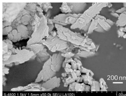
Fig. 2. Electron microscope image of particles formed in the cooling water for electromagnets and RF cavities at the J-PARC MR facility.
