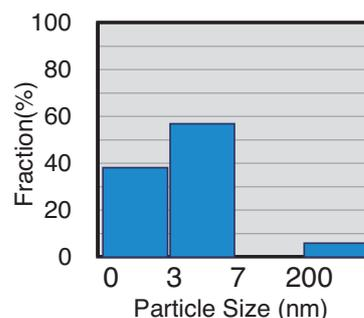
Fig. 1. Non-colloidal (0–3 nm) and colloidal fractions for different size ranges (3–7, 7–200, and >200 nm) of  $^7\text{Be}$  in the cooling water for electromagnets at the 12 GeV proton accelerator facility, KEK.
