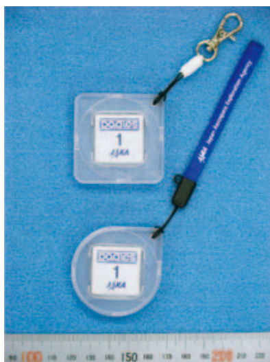
Fig. 1. Area PADLES for area radiation monitoring (upper) and Crew PADLES for personal dosimetry (lower).
