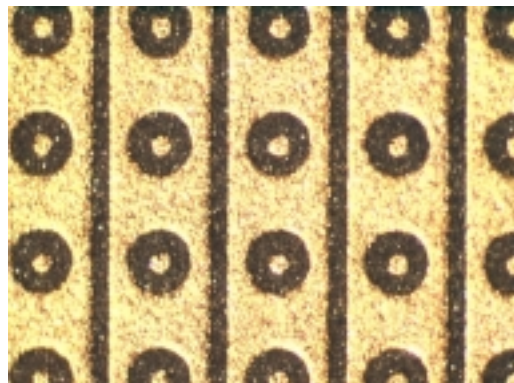
Figure 2: Close up view of detection area of the \mu -PIC.
