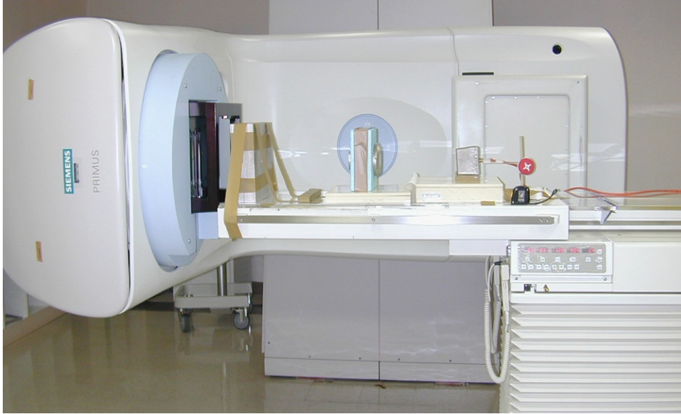
Fig. 1. Setup for monitor chamber backscatter measurement.
