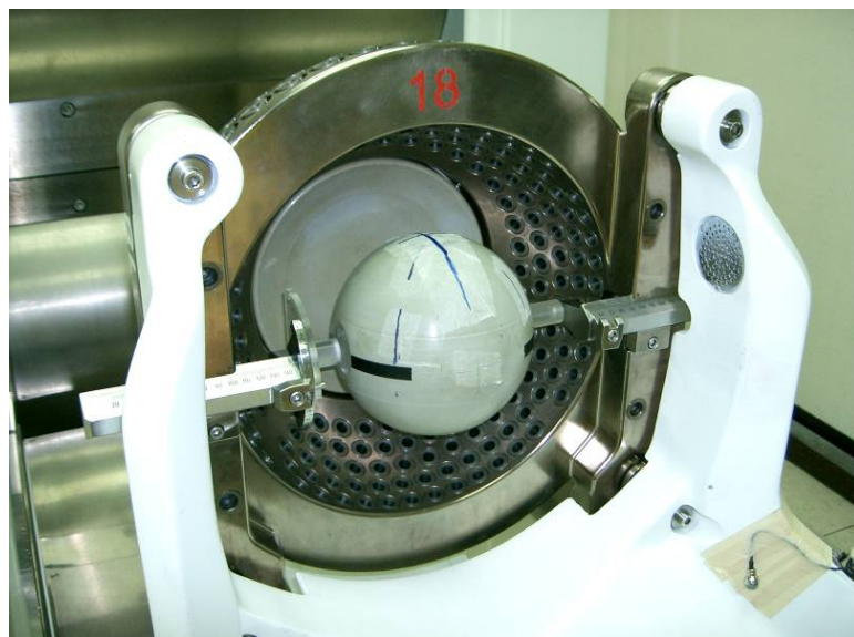
Figure 2. Spherical phantom was mounted at the unit center point position ( x=y=z=100 mm) with in the 18mm collimator helmet.
