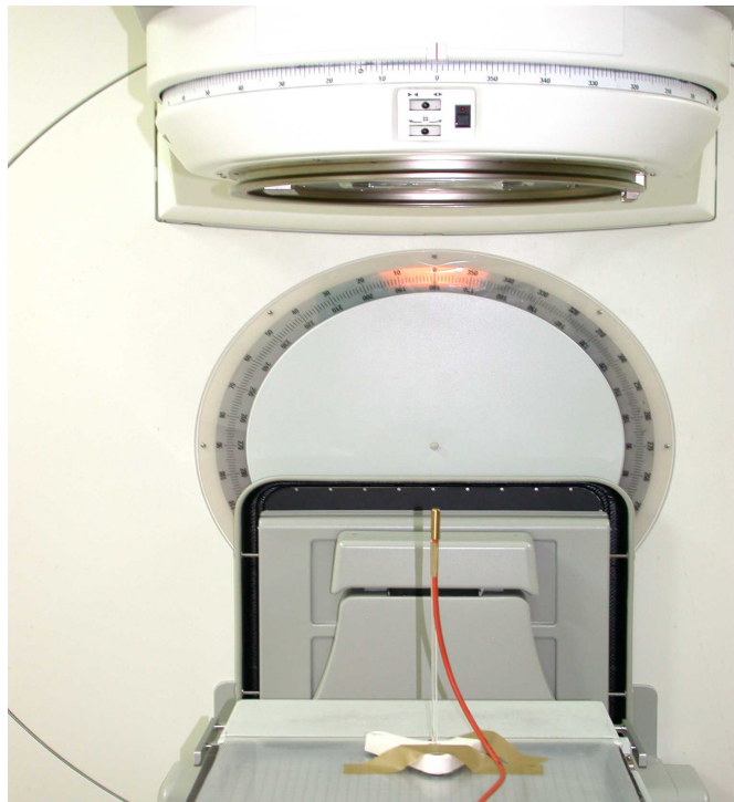
Fig.2. The setup method of in-air output factors measurement.
