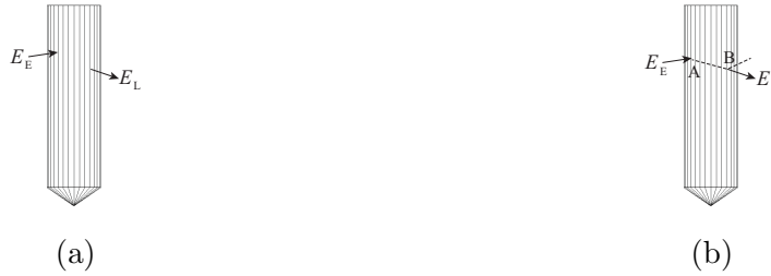
Figure 4: (a): E_E Electron energy entering in the detector. E_L Electron energy leaving from the detector. Detection volume is filled with air or water. (b): The electron with E_E had caused bremsstrahlung at A and the generated gamma-ray caused a Compton scattering at B. Dashed line shows a gamma-ray.
