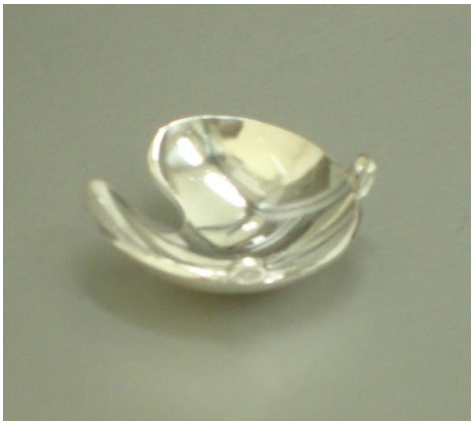
Figure 1. Picture of a COC type Ru-106 source (a) and schematic drawing of the cross section (b). The solid curve in the gray colored region in (b) refers to a radioactive layer. Geometric parameters of the CCB and COC type sources are 20.2 mm and 25.4 mm in diameter D , 12 mm and 14 mm in radius R , and 5.4 mm and 7.5 mm in height h , respectively.
