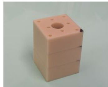
(b) Laminated phantom simulating a mouse
