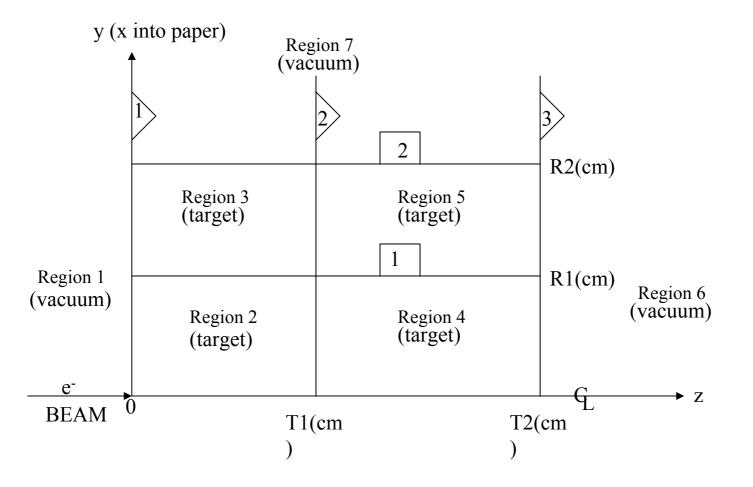
**Subroutine CYL2** : Treats particles between 2 cylinders This subroutine corresponding to PLAN2P for the two parallel planes.
